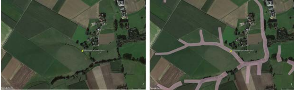
Figure 23. Detail of Maarkebeek catchment in Belgium with visible likely (permanent) gully (left); detail prediction of location of ephemeral gullies and suitable locations for grassed waterways (right).
